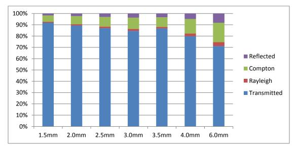
Figure 3: The scattered photons for Al at 80kV
