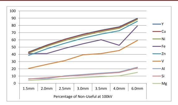
Figure 10: Calculated data for the Non-useful photons for 100 kV
