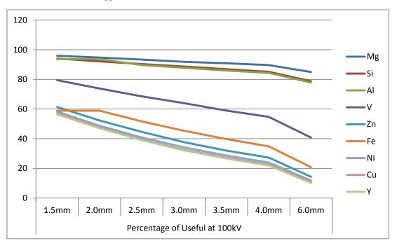
Figure 7: Calculated data for the useful photons for 100 kV
