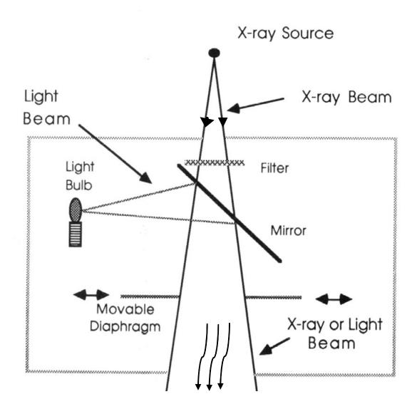
Figure 1: A Typical design of an X-ray source showing the filter (Jan Kybic, 2006)
