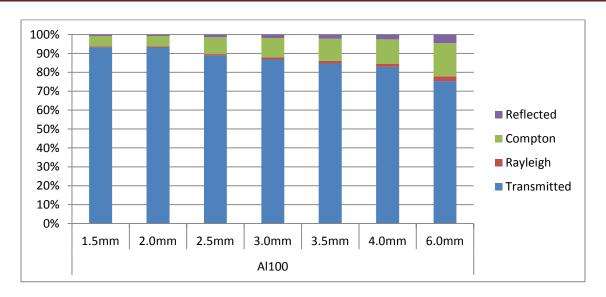
Figure 4: The scattered photons from Al at 100 kV
