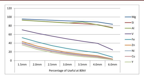
Figure 6: Calculated data for the useful photons for 80 kV
